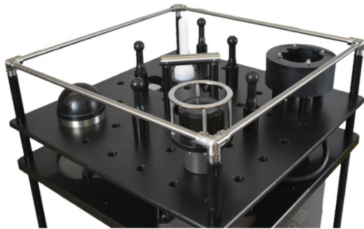
Possible configuration of 5 hydrophones and 3 communication transducers
